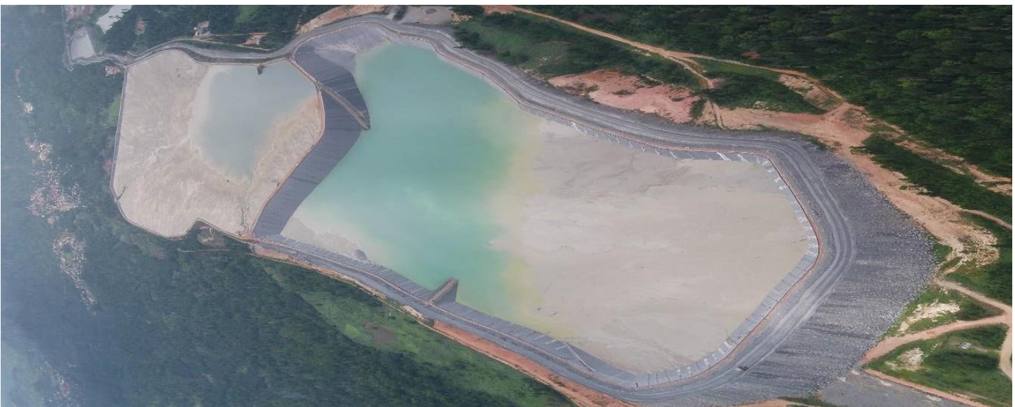
Newmont Goldcorp’s Akyem Mine TSF Cell 1 (Left) and TSF Cell 2 (right), Ghana, Downstream Construction. 23
